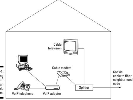
Figure 6-1: Connecting VoIP through a cable modem.
